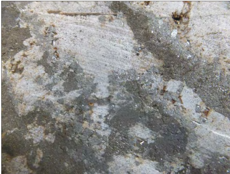
Figure 7-6 Quartz and arsenopyrite (silvery gray) cut by pyrrhotite (dark veinlet, upper right), SM19-014, 468 ft (Sillitoe, 2019)
