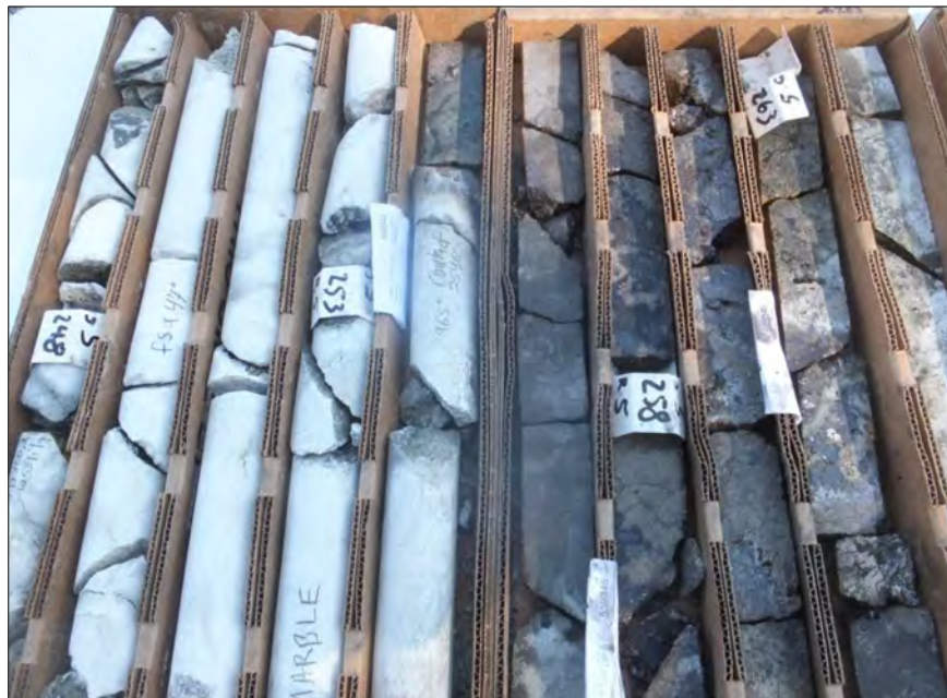
Figure 7-5 Massive sulphide replacing Laxey Marble, SM19-003, 248-263 ft (Sillitoe, 2019)
