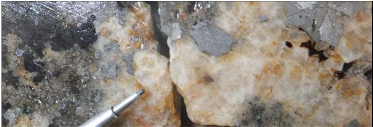
Figure 7-7 Quartz-arsenopyrite (right) in contact with massive sulphide (left), SM19-003, 209 ft (Sillitoe, 2019)
