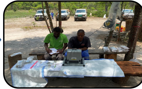
3. Field pXrf Laboratory analyze samples onsite for real-time data.
